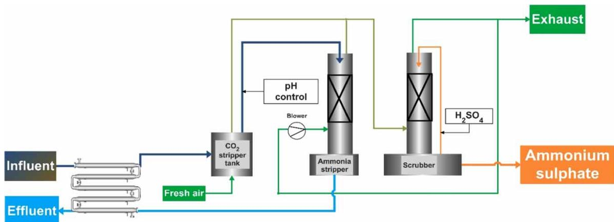
**Figure 1** | Schematic overview of the demonstration plant.
