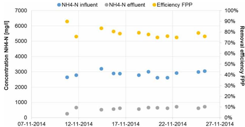
Figure 2 | Influent and effluent concentrations NH<sub>4</sub>-N and removal efficiency.
